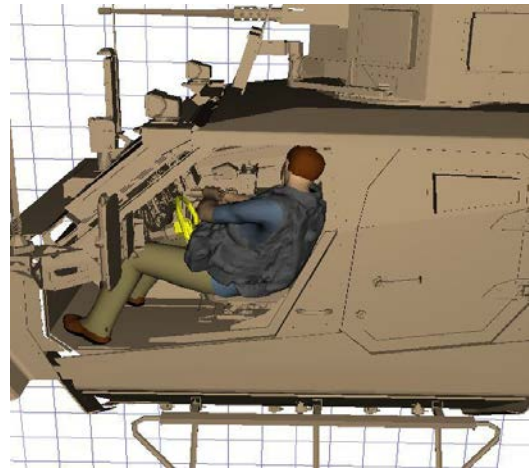
Figure 5. Large-male encumbered manikin in the intermediate position for assisted incapacitated egress.
