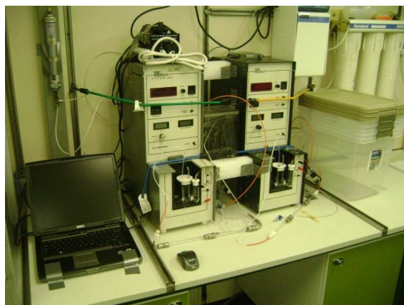
Figure 8: UIC coulometer in the shipboard lab.
