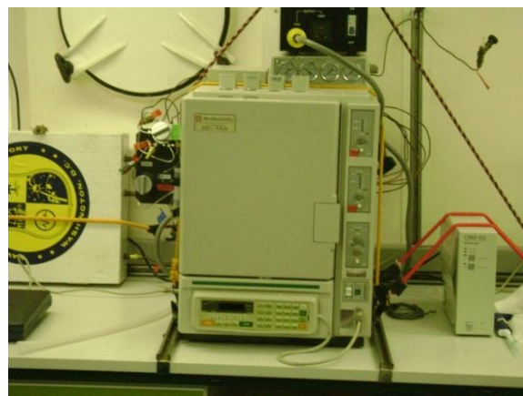
Figure 9: GC-FID Shimadzu GC-14A gas chromatograph in the shipboard lab.
