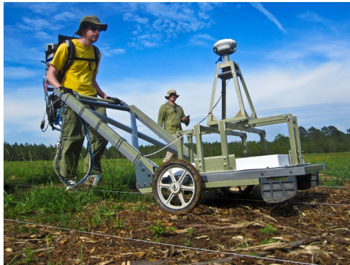
Figure 5-3 – TEMTADS MP 2x2 Cart with GPS Antenna Tripod. Photograph by Harry Wagner.
