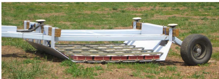
Figure 5-5 – Sensor array mounted on the MTADS EMI sensor platform.
