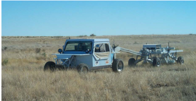
Figure 5-2 – MTADS tow vehicle and magnetometer array.
