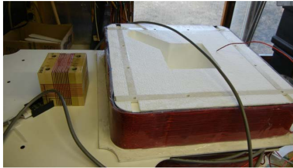
Figure 2-5 – Individual TEMTADS/3D EMI sensor with 3-axis receiver under construction.
