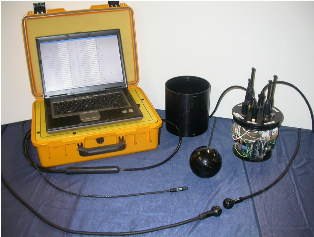
Figure 2: Acoustic communication system hardware (with the high-power source transducer Jetasonic H320).
