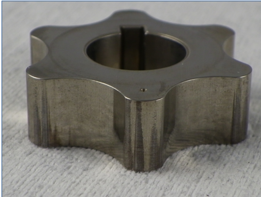
Figure G-16. Transfer Pump Gear
