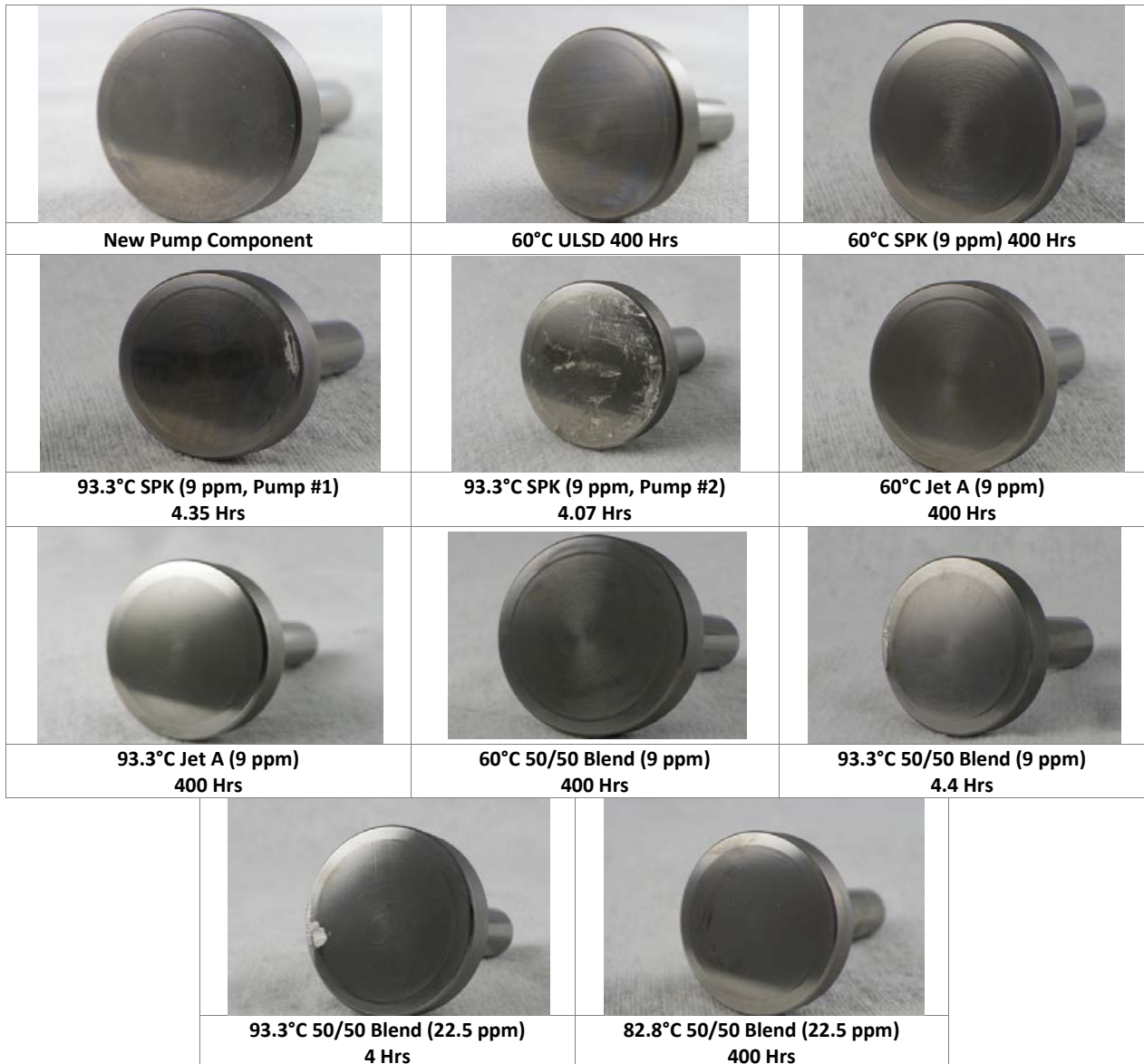
Figure 28. Lower Plunger Face
