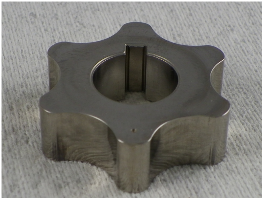
Figure D-13. Transfer Pump Gear
