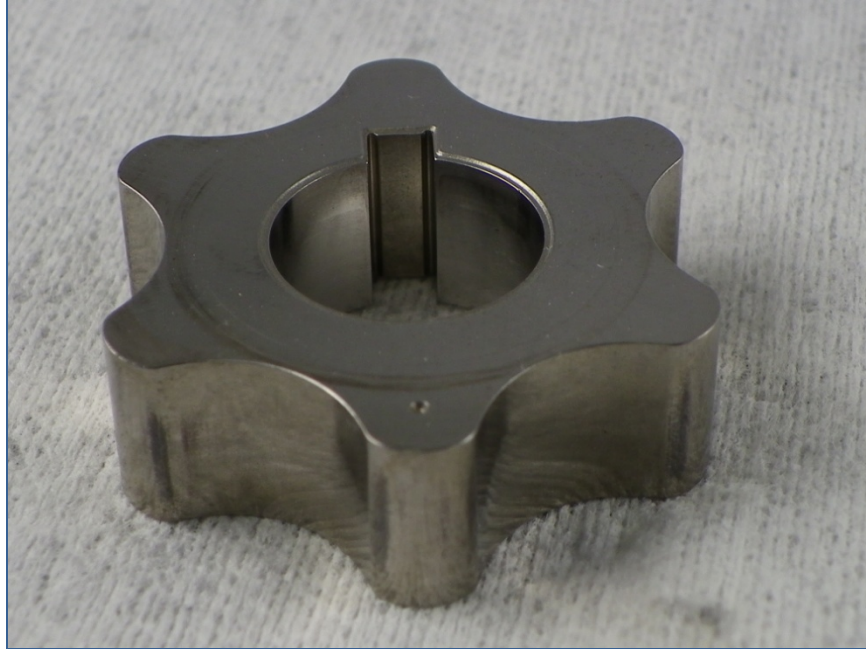
Figure E-14. Transfer Pump Gear
