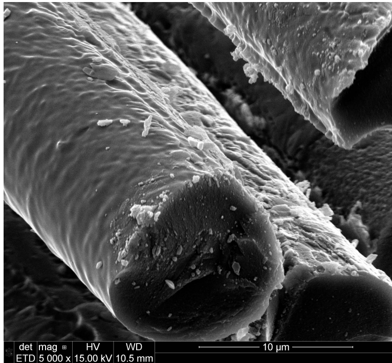
Figure 7.208: Hi-Nicalon S fiber specimen S47, tested in steam at 1000°C at 255MPa
