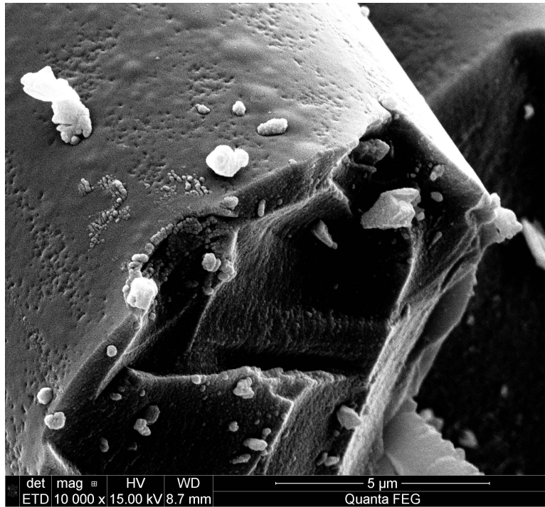
Figure 7.182: Hi-Nicalon S fiber specimen S38, tested in steam at 900°C at 353MPa
