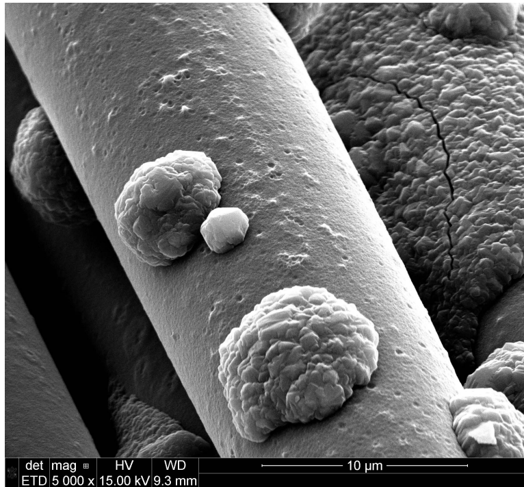
Figure 7.91: Hi-Nicalon S fiber specimen S50, tested in steam at 800°C at 353MPa
