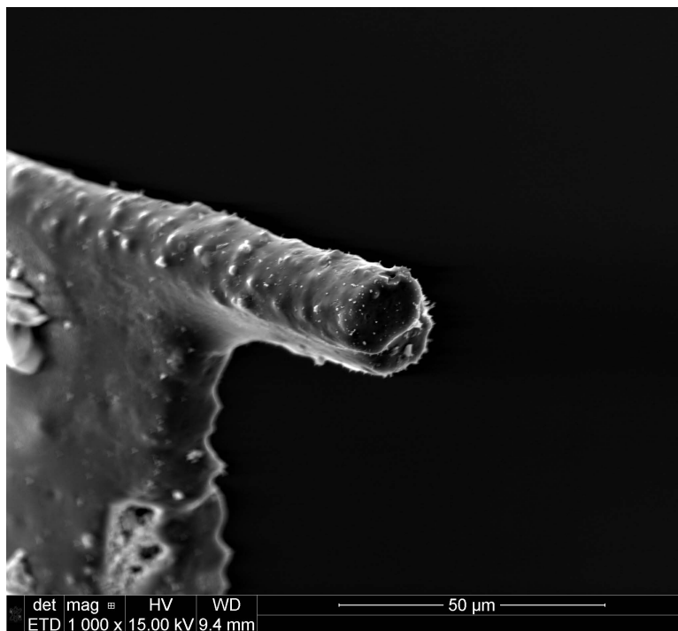
Figure 7.104: Hi-Nicalon S fiber specimen S21, tested in steam at 800°C at 400MPa
