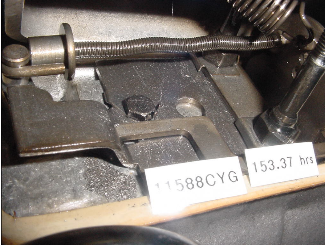
Figure 4. Metal Debris inside Pump at 153-hours for Test No. 4
