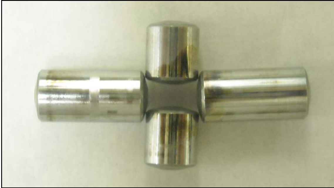
Figure 14. Delphi Pumping Plunger Wear Scars after Operation with S-8/Jet A + 22.5 ppm DCI-4A Fuel
