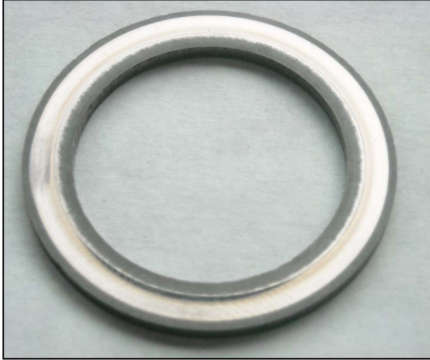
Figure 13. Delphi Thrust Washer with Typical Wear Pattern after 500 hours Jet A Fuel
