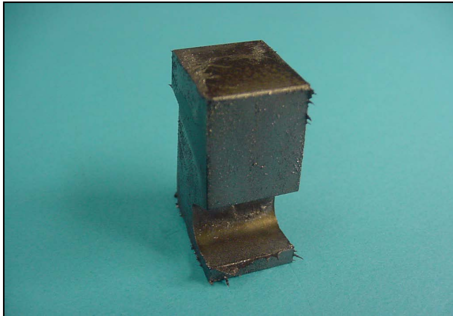
Figure 9. Delphi DPA Pump Governor Weight with 50/50 S-8/Jet A Fuel with 22.5-ppm DCI-4A CI/LI Additive
