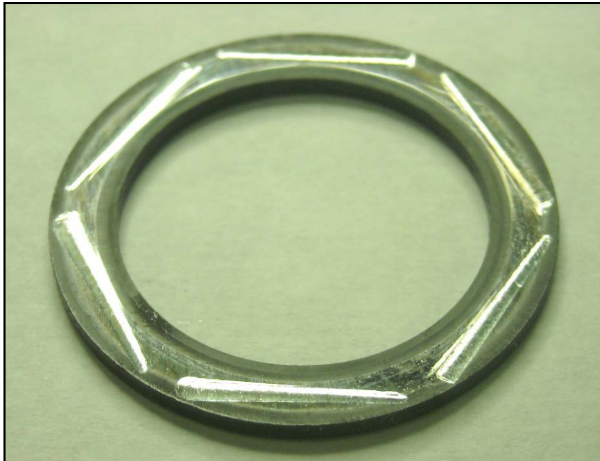
Figure 12. Wear Scars on Governor Thrust Washer from Governor Weights at 250 hours with S-8/Jet A + 22.5 ppm DCI-4A Fuel
