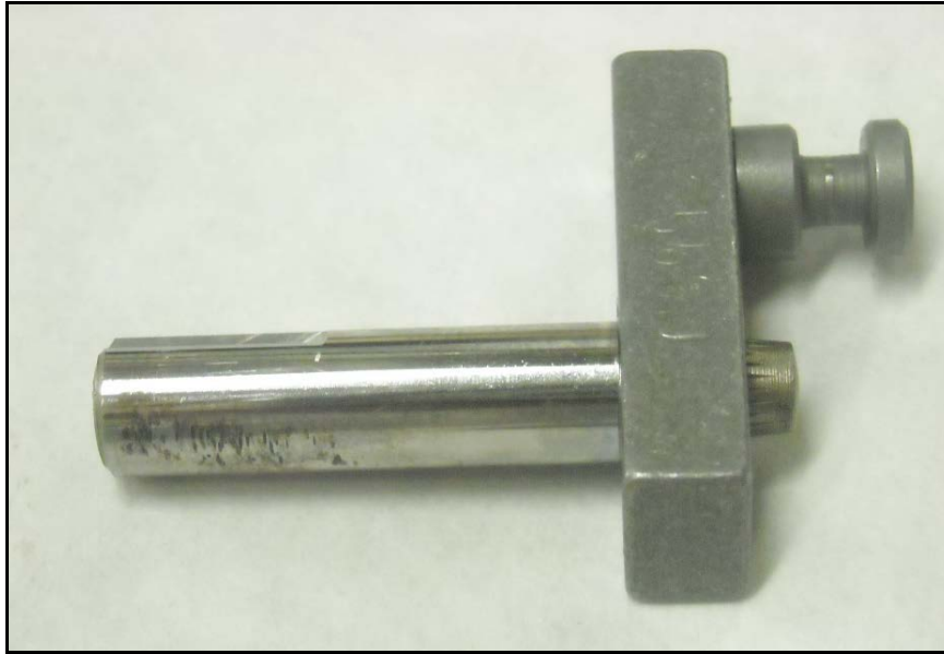
Figure 11. Delphi Rotary Fuel Injection Pump Metering Valve after 250 hours with S-8/Jet-A + 22.5-ppm DCI-4A Fuel
