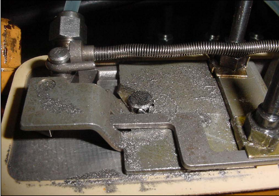
Figure 2. Delphi Pump Wear Debris with S-8 (F1000) Fuel
