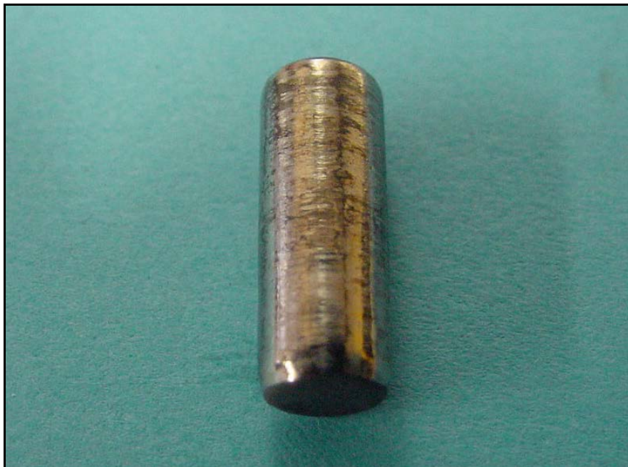
Figure 7. Delphi DPA Pump Cam Roller Wear with 50/50 S-8/Jet A Fuel with 22.5-ppm DCI-4A CI/LI Additive
