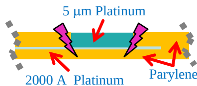
Figure 7. Mechanical mismatch causes stress at the electrode boundaries. Schematic illustrating electrode instability.
