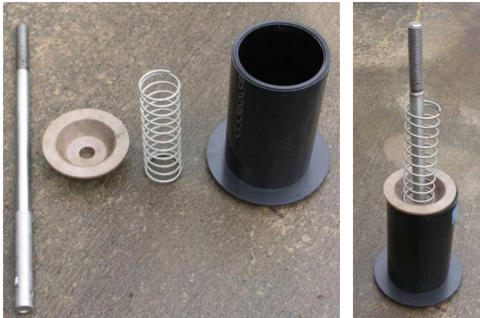
Figure 4. DATV stainless steel stem, brass valve, stainless steel spring, and barrel sleeve separately (left) and mocked up as assembled (right).
