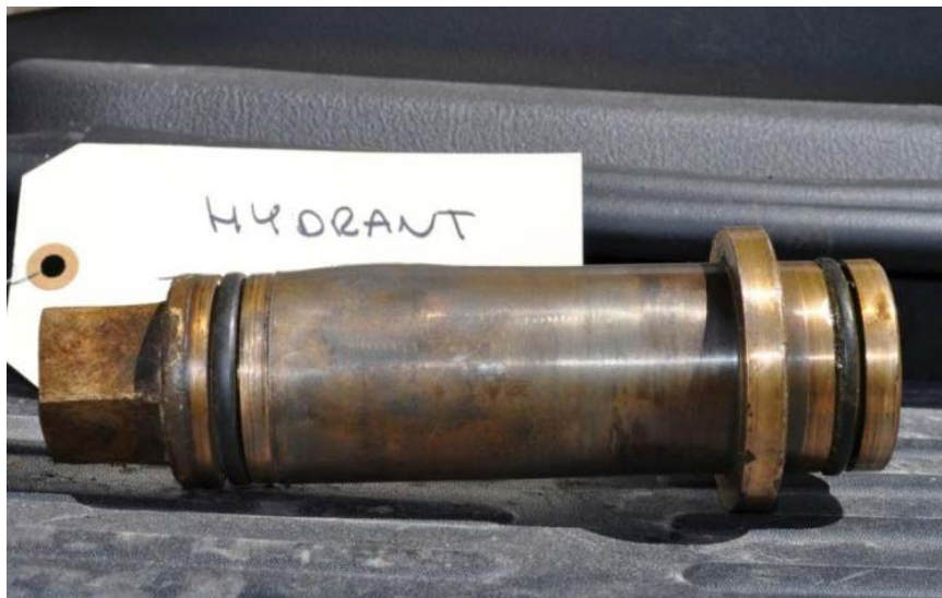
Figure 24. Bulge in operating nut sleeve.
