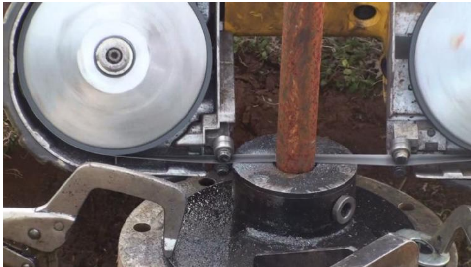
Figure 8. Cutting the solid stem.
