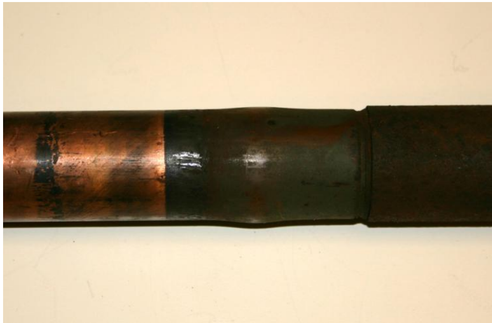
Figure D1. Fire hydrant valve stem showing bulge in copper sleeve.
