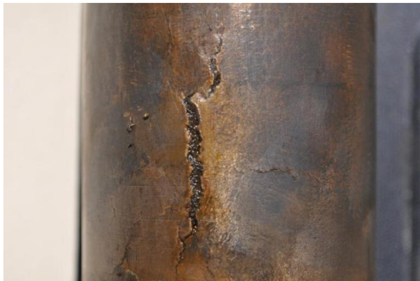
Figure 23. Operating nut sleeve* showing cracks due to freezing water trapped inside the barrel.
