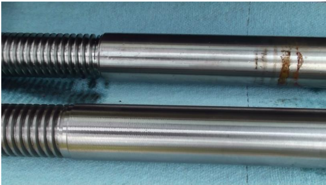
Figure 19. Cold-rolled stem design as supplied by manufacturer (Mueller Standard) with zero days of use (left) and 12 months exposure (right).
