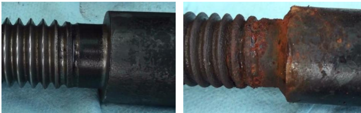
Figure 19. Cold-rolled stem design as supplied by manufacturer (Mueller Standard) with zero days of use (left) and 12 months exposure (right).
