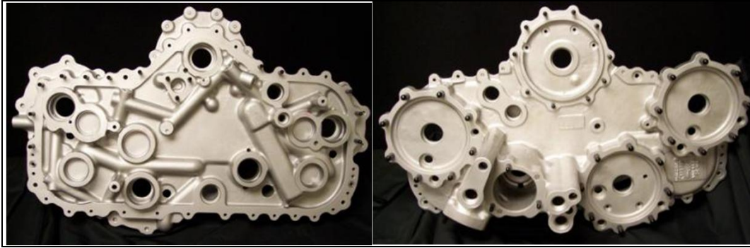
Figure 59. H-47 accessory cover after media blast cleaning.
