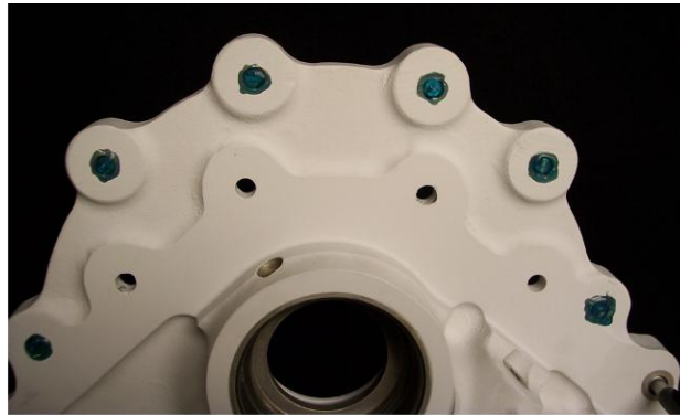
Figure 64. Example of UV curable maskant on stud bottoms of H-47 accessory cover.
