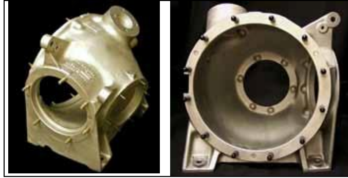
Figure 16. H-60 gearbox housing after media blast cleaning.
