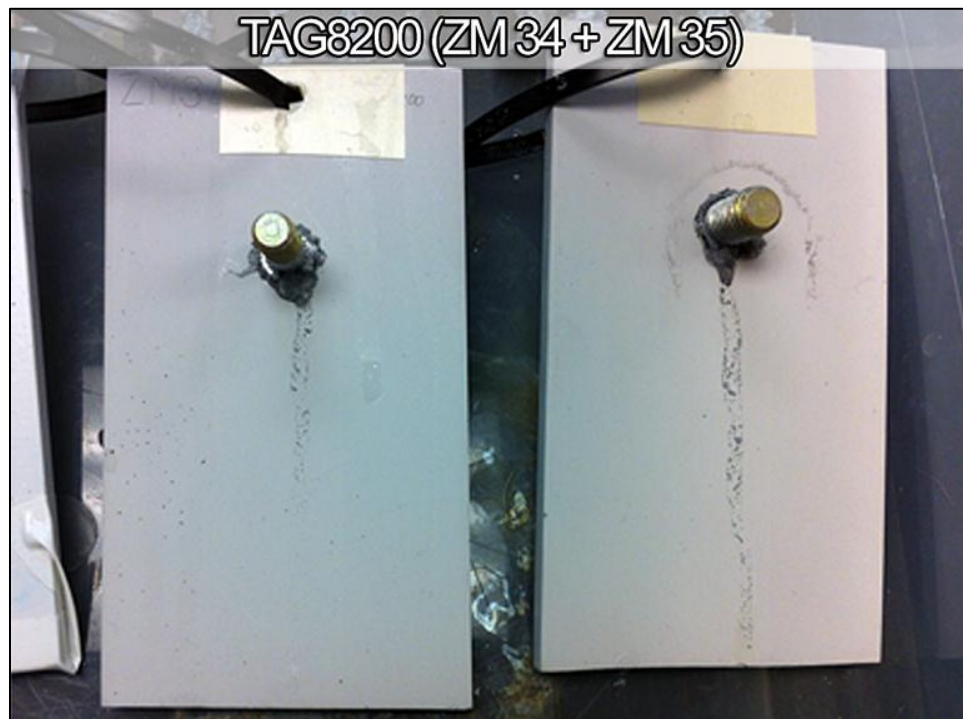
Figure 34. TAG8200 panels after 16 hrs of B117 test.
