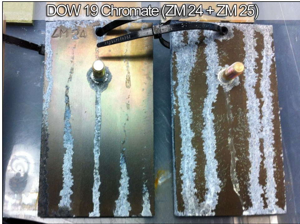
Figure 36. DOW19 Chromate panels after 16 hrs of B117 test.
