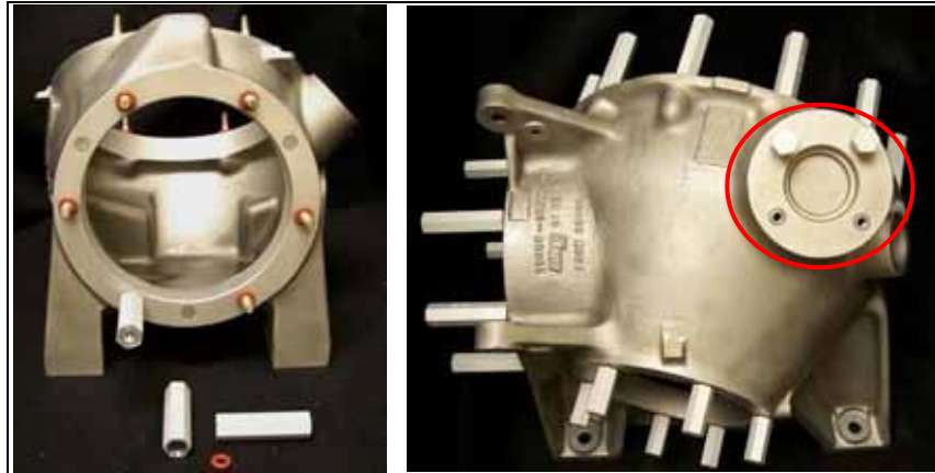
Figure 18. Masked H-60 components. Left: aluminum stud covers on center housing, right: stud covers and helicoil covers (red) on gearbox housing.
