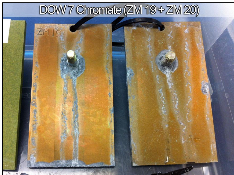
Figure 35. DOW7 Chromate panels after 16 hrs of B117 test.
