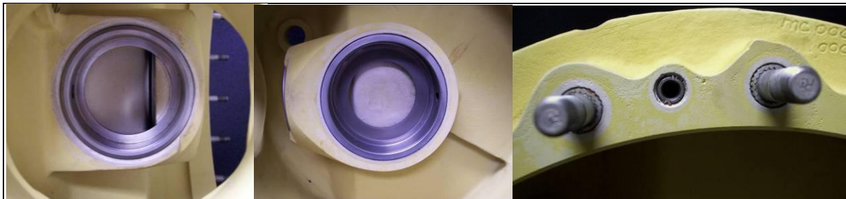
Figure 37. H-64 tail rotor gearbox housing after Brush Tagnite touchup around mixed metal inserts.
