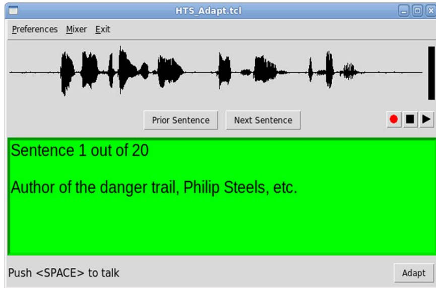
Figure 7: Screenshot of the GUI Used to Record Sentences and Adapt an HMM-Based Speech Synthesis System
