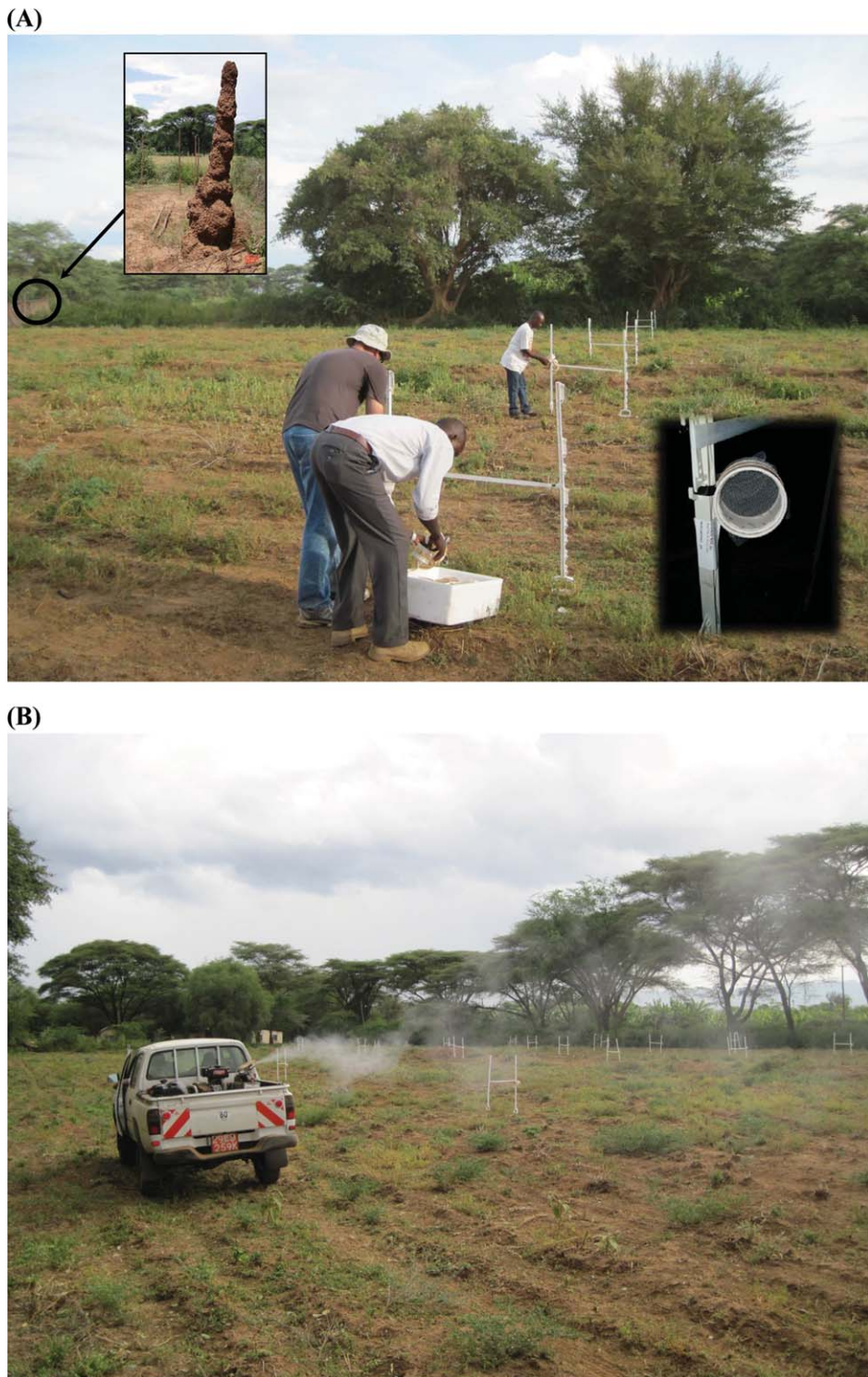
Fig. 2. (A) Sentinel sand fly cages being removed from coolers and affixed to posts in the west plot on the second spray day; looking south. Cotton droplet capture ribbons have already been attached in position between the posts at each cage position. Upper left inset shows approximate location of one of the termite mounds (2.5 m high); lower right inset shows close-up of sentinel cage and adjacent cotton ribbon attached to pole. (B) View of the west plot on the second spray day showing the sand fly cages and droplet capture ribbons in position, with the Terminator ULV being operated from a truck bed; looking north west.
