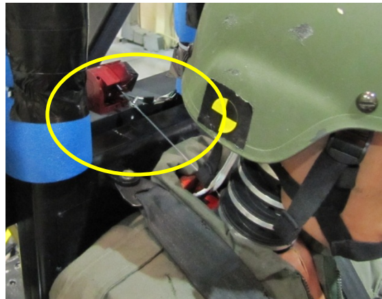
Figure 10. Neck Displacement Transducer
