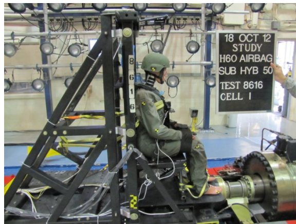
Figure 1. AFRL HIA Shown with Rigid Seat Configuration
