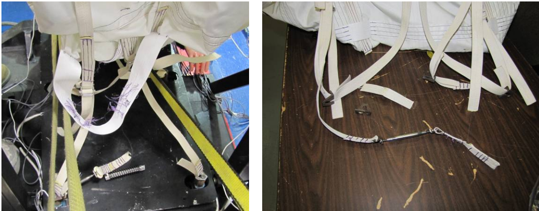
Figure 29. HIA8708 Broken webbing tensioners
