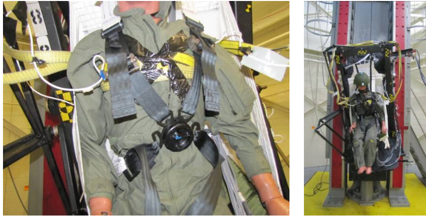
Figure 8. VDT6288 (L) Restraint Buckle post-test (R) Manikin position post test
