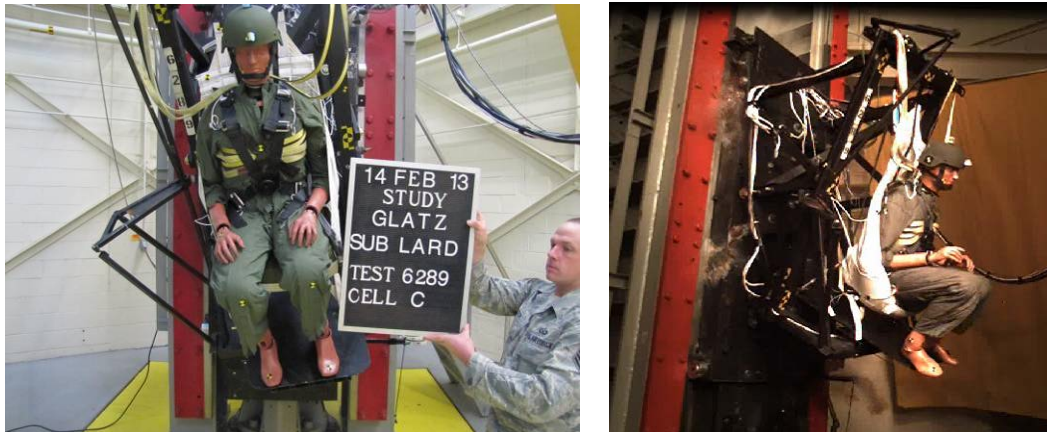
Figure 9. VDT6289 (L) Manikin initial position (R) Seat ripping during test
