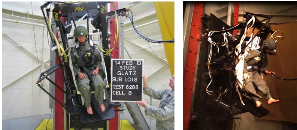
Figure 7. VDT6288 (L) Manikin position pre-test (R) Manikin rebound after initial pulse
