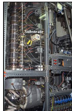
Figure 4 – One of two Cylindrical Magnetron Sputtering platforms for short length, large caliber gun barrels.
