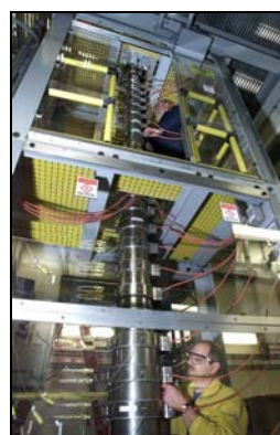
Figure 5 – Full-length, pre-production Cylindrical Magnetron Sputtering Platform for large caliber gun barrels.
