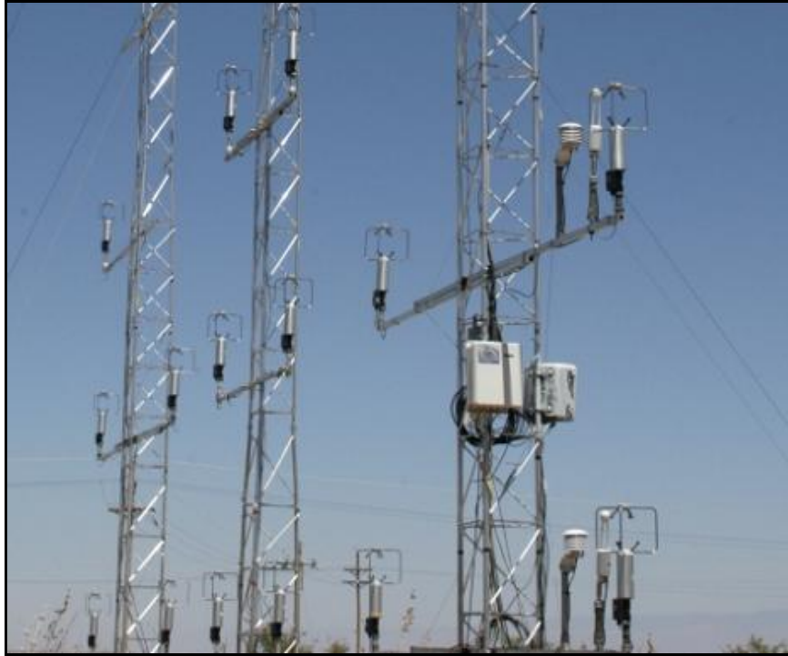
Figure 5. View of lowest tower array level, Li-Cor hygrometer electronics boxes and 2 m and 4 m “fetch” array levels on right (south) of tower array.
