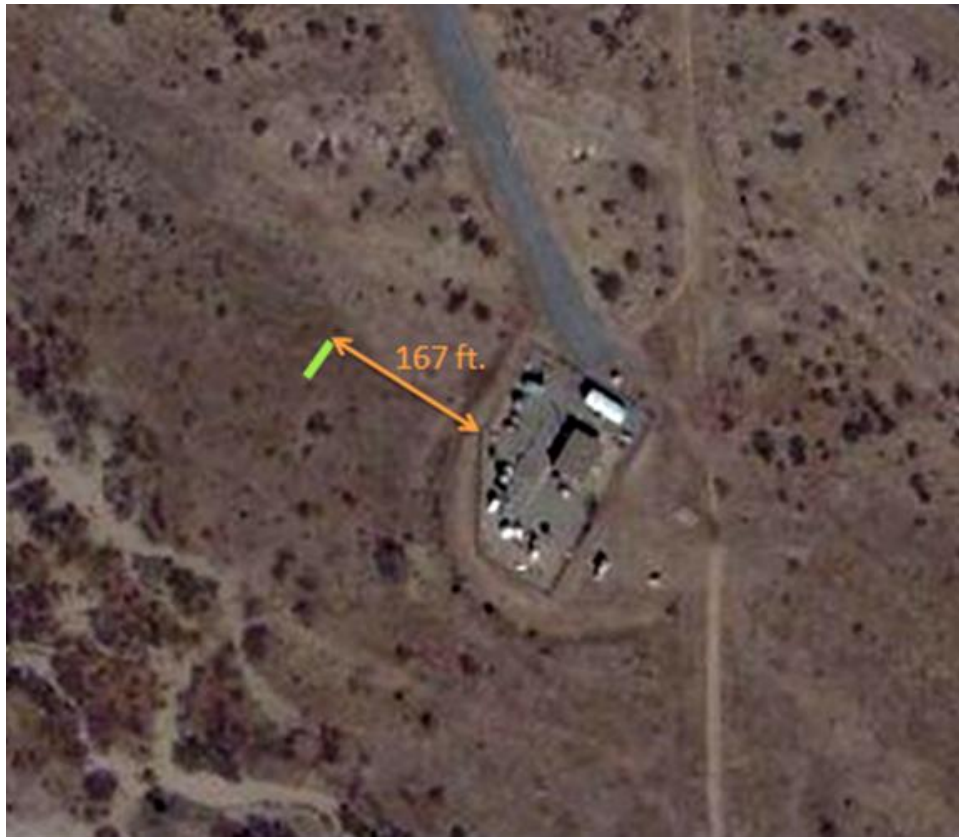
Figure 2. Building 19472 compound on WSMR, NM, its near environs, and the approximate location and orientation of the two-dimensional array 167 ft. away relative to the compound fenceline.
