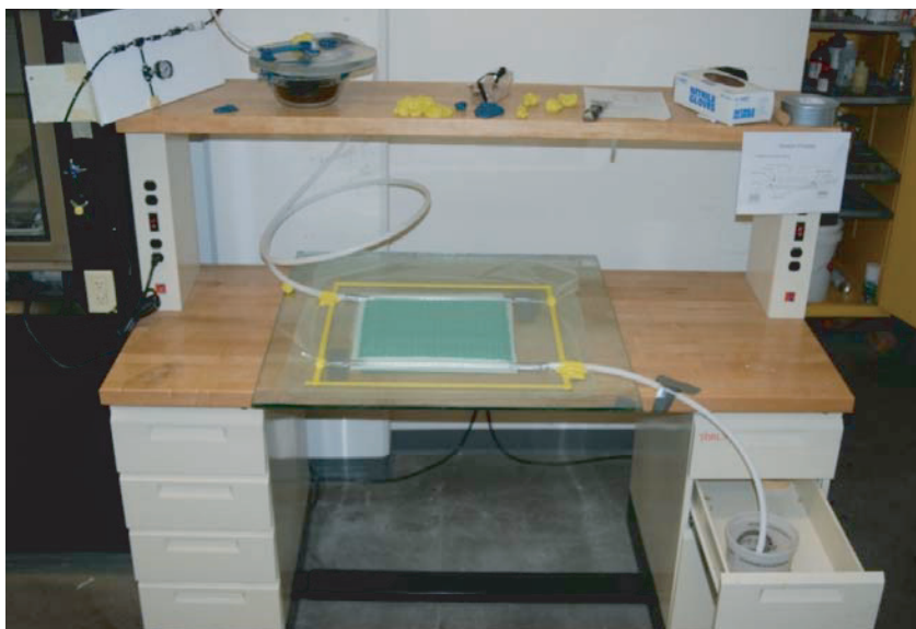
Figure 2. Fabrication of samples using the VARTM process.
