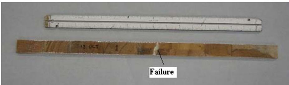
Fig. 22 Typical failure under wet impact at the impact site
