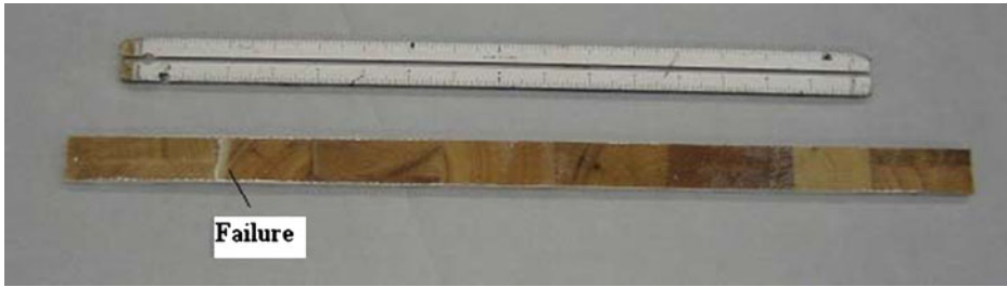
Fig. 21 Typical failure under dry impact at the boundary edge
