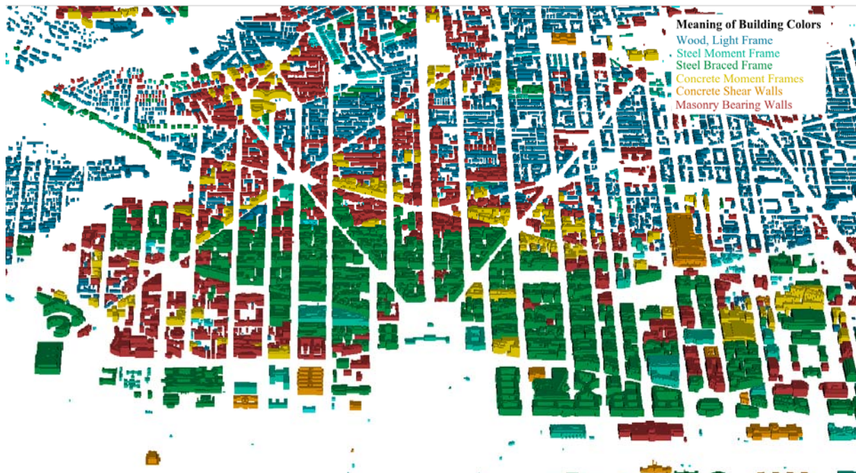
Figure 2-1. Washington, D.C. represented on a 3-D lattice model. The different colors correspond to different Hazus building types.
