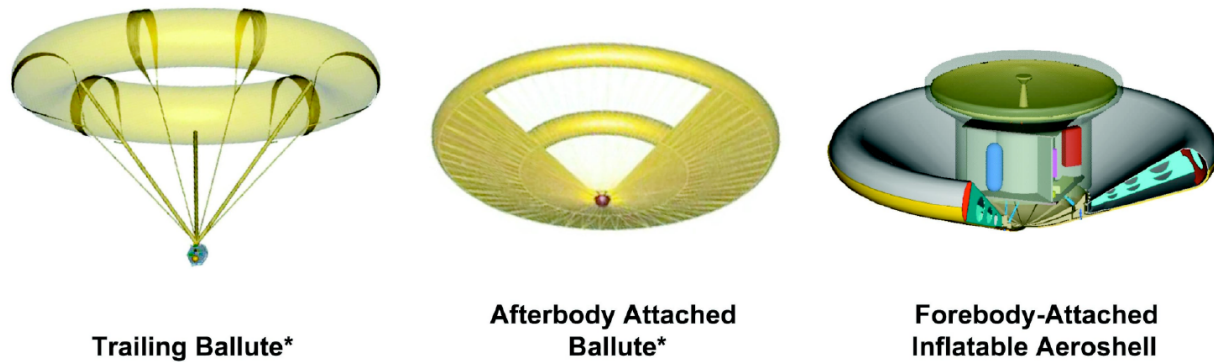
Figure 6: Typical Inflatable Aerodynamic Decelerators (IAD) [18]
