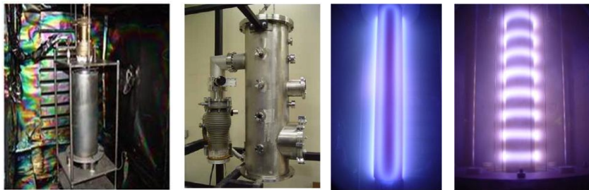
Fig. 4c Biased DCMS and HIPIMS cylindrical sputter deposition systems at Southwest Research Institute, showing two target designs- left used rectangular magnet, right used ring magnet.
