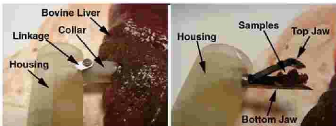
Figure 7. Ex vivo tissue sample collection (left) and multiple tissue samples shown in biopsy grasper after sampling (right).
