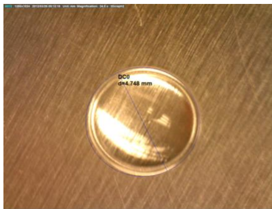
Figure 28. A 10 \mu\text{L} droplet of EG75 with a diameter of 4.748 mm.
