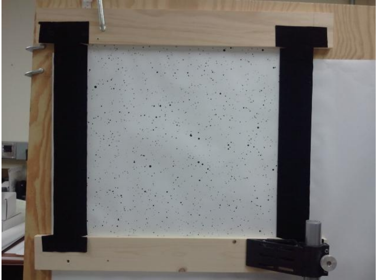
Figure 12. VLSTRACK witness card 15 on mounting frame.
