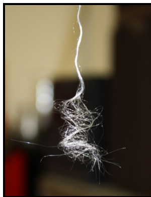
Figure 16. Fibril Fracture Mode of Individually Tested Drop Yarns
