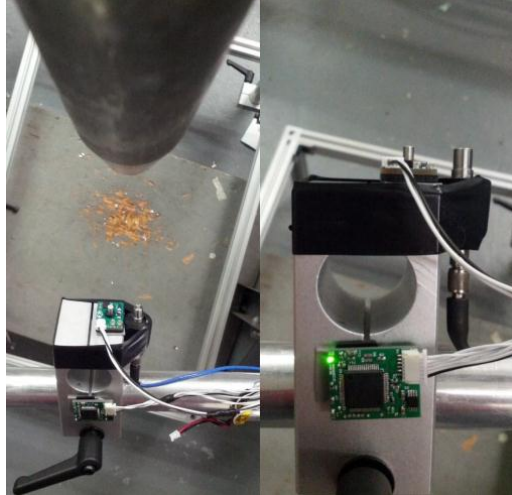
Figure 3 (a): Location of the CBI-ESP sensor board (right) relative to the witness sensor (PCB Piezotronics)
