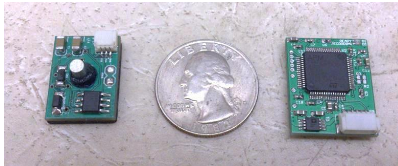
Figure 2 Real size of CBI-ESP sensor and DAQ board
