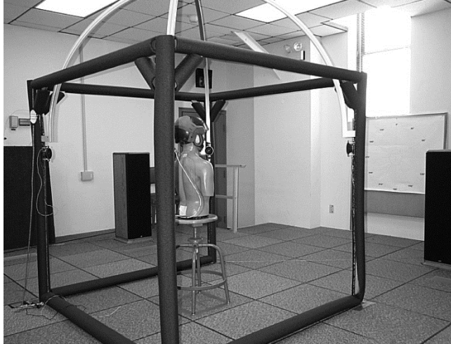
Figure 3. The loudspeaker array used for sound presentation.
