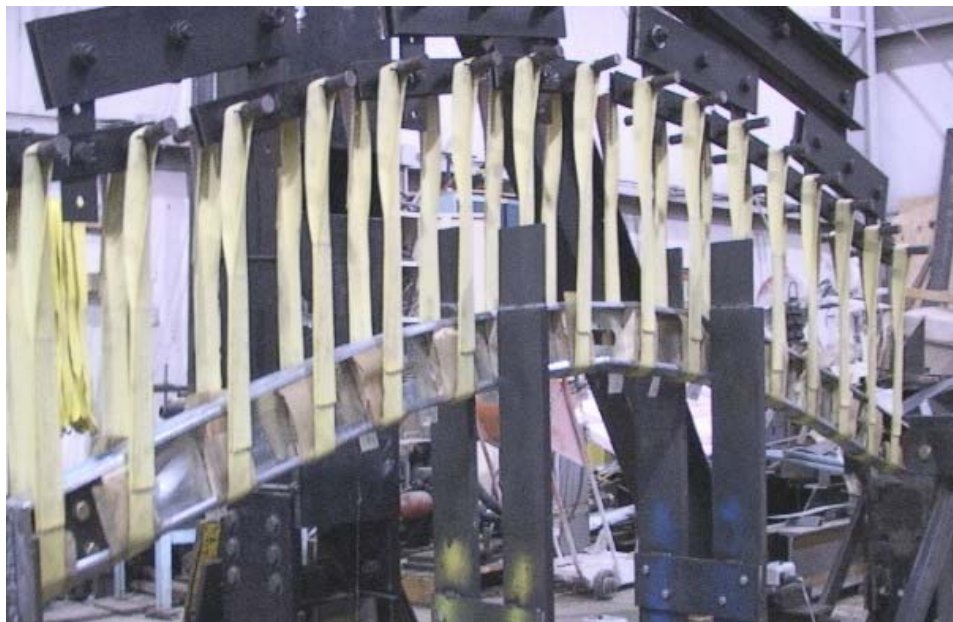
FIG. 4. Loading tree component test Setup
