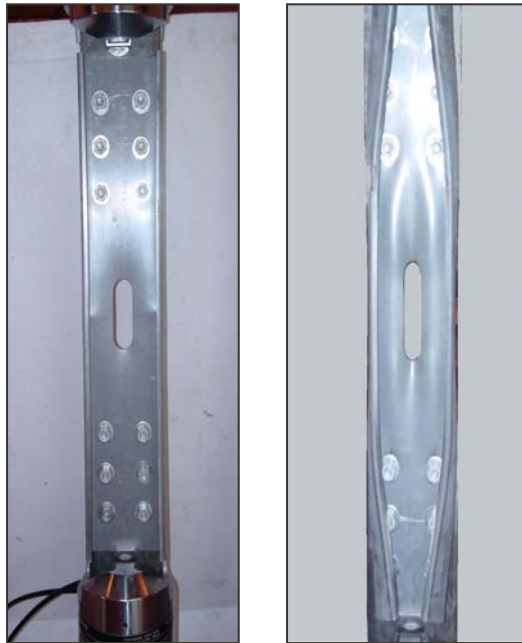
FIG. 2. Steel stud specimen loaded in tension; note six bolts were required to yield the steel stud cross-section
