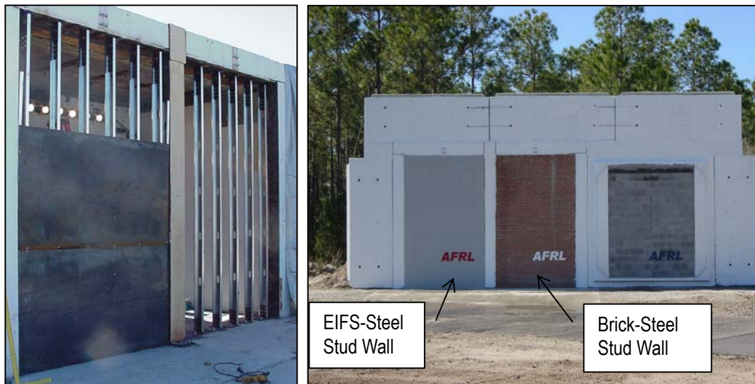
FIG. 9. Pretest exterior photo of BREW-1 structure showing EIFS and brick façade on steel stud walls anchored using blast-resistant connection design; walls during construction (left)
