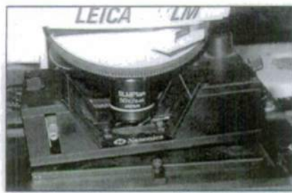
Figure 1. A SPM/NSOM/Confocal system attached to a spectral imaging system. (SPM, Nanonics Imaging Ltd.). This system is configured with nanoindentation and scratch capability. (Nanonics)
