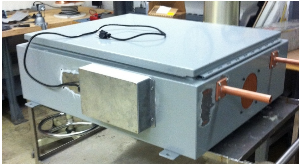
Figure 240. RF enclosure for model 40168
