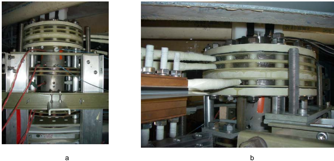
Figure 107. (a) New Guide and Mirror coil set; (b) close-up of upper mirror coils and clamping structure
