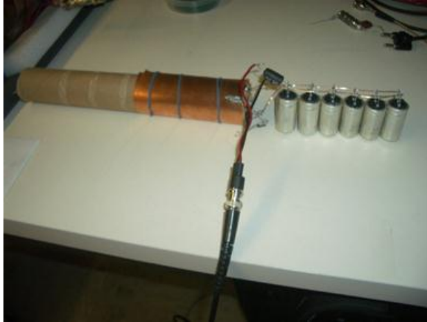
Figure 278. Close-up of mock-up bank to characterize resonance for deriving inductance
