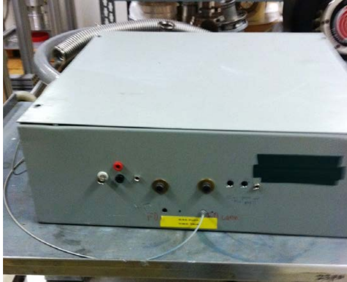
Figure 219. Gas-puff driver enclosure
