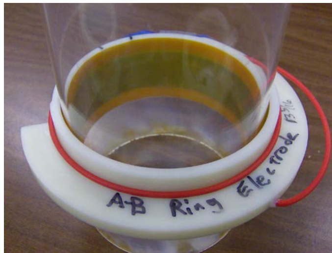
Figure 236. Electrode assembly surrounding quartz tube
