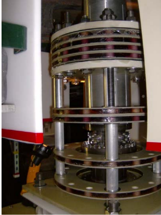
Figure 73. Guide and Mirror coil structure with new clamping assembly on each side of upper coil set
