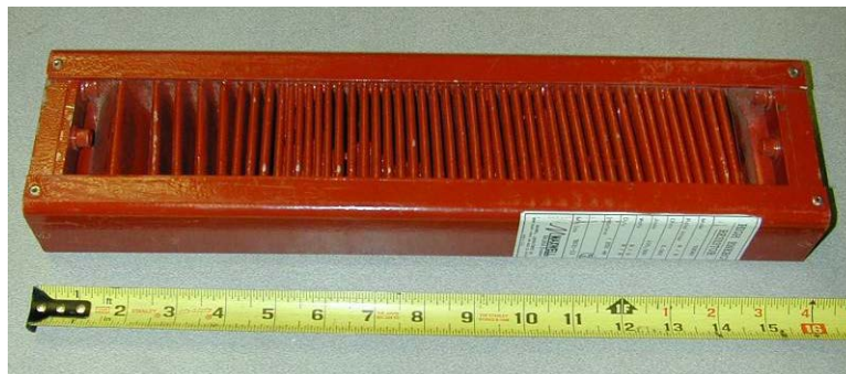
Figure 98. A 0.060-Ω Franklin resistor, shown with a tape measure for scale
