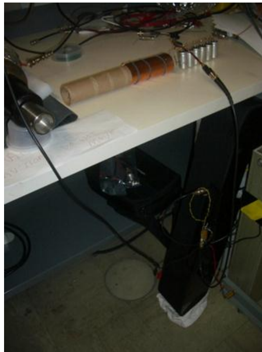
Figure 277. Bench mock simulation of Ring bank capacitance and inductance with 50-W amplifier
