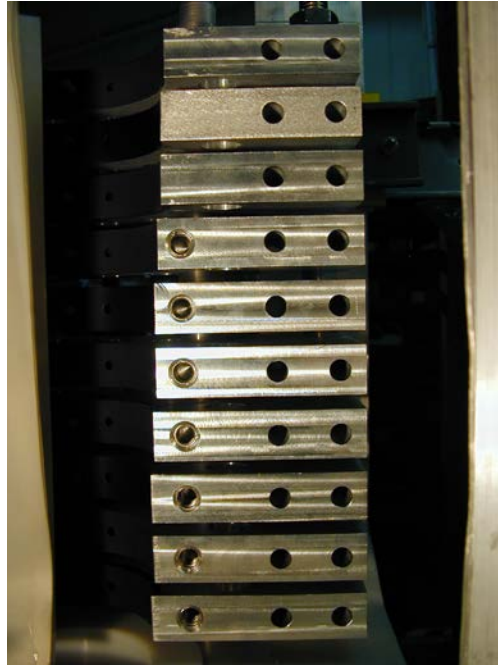
Figure 128. Current-joint surfaces of Theta coil segments left assembled on vacuum stand
