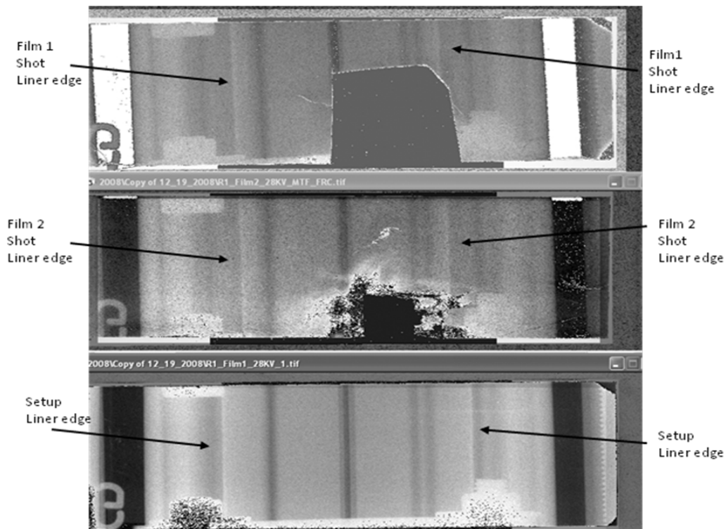
Figure 47. Images from X-ray #1 imaging system (top and middle); setup image taken before the shot (bottom)
