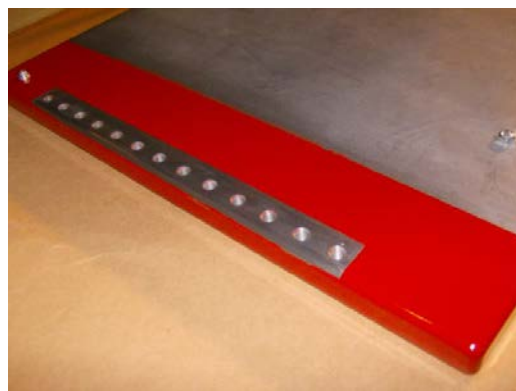
Figure 151. Painted end of PI hot bus plate, where rail-gap switch is mounted
