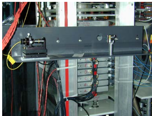
Figure 184. Fiberglass platform supporting the receive fiber coupler and its turning mirror
