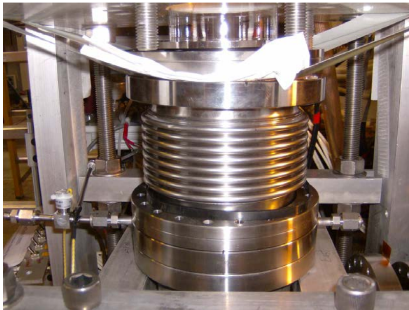
Figure 221. Puff-valve assembly mounted on the experiment
