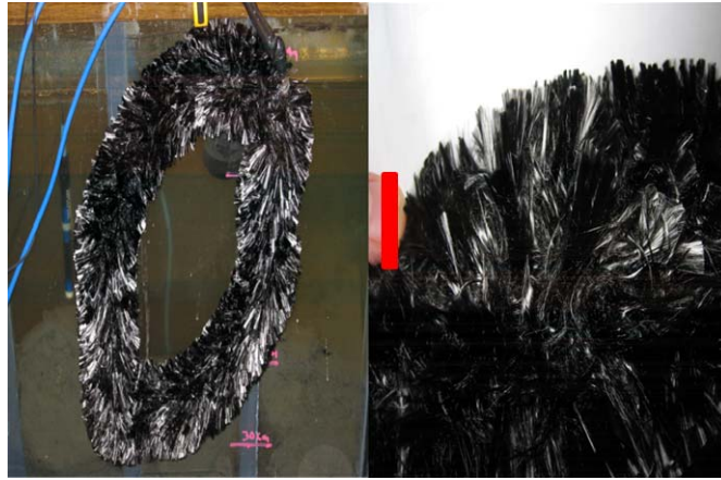
Figure 5. Left: Graphite carbon bottle brush connected to the conducting wire, Right: Upclose image of large surface area created by the individual conductive graphite fibers. Red scale bar is approximately 2 cm.
