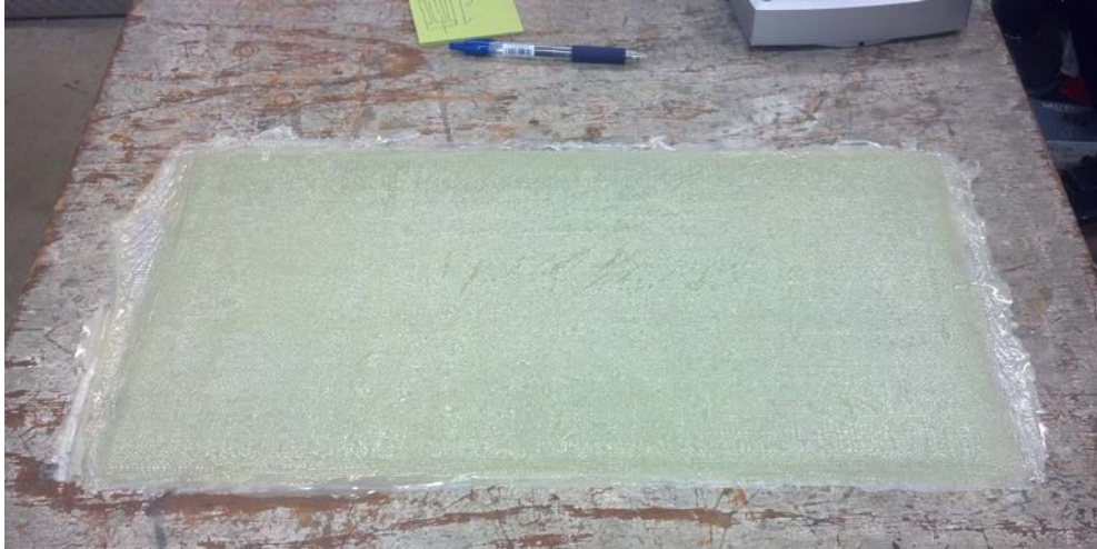
Figure 4. Beam Sample Prior to Cutting into Strips
