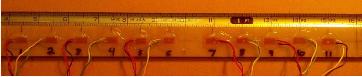
Figure 10. Beam Strain Gage Orientation
