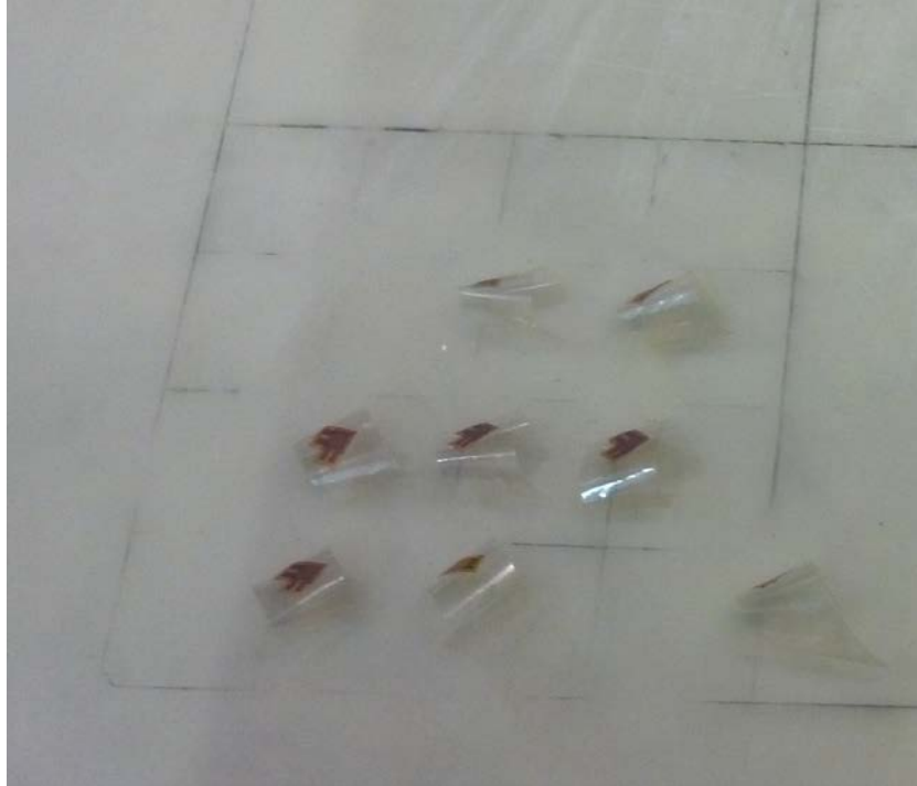
Figure 6. Taped Strain Gages, Prior to Being Affixed to Sample.
