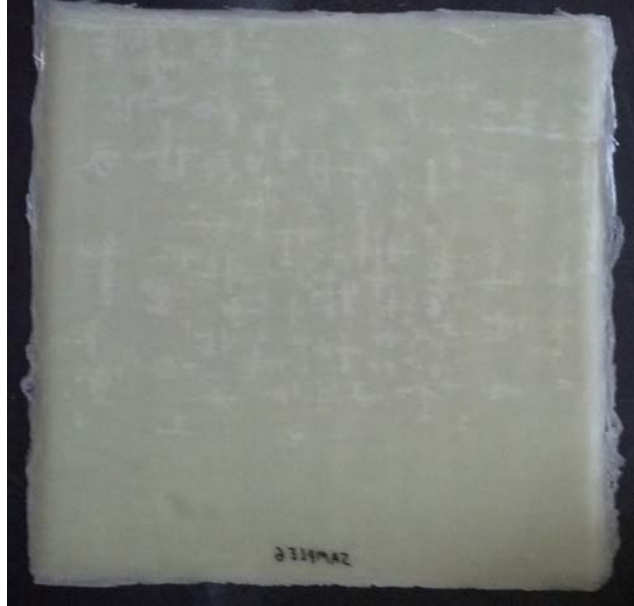
Figure 3. Dry Patches Due to Vacuum
