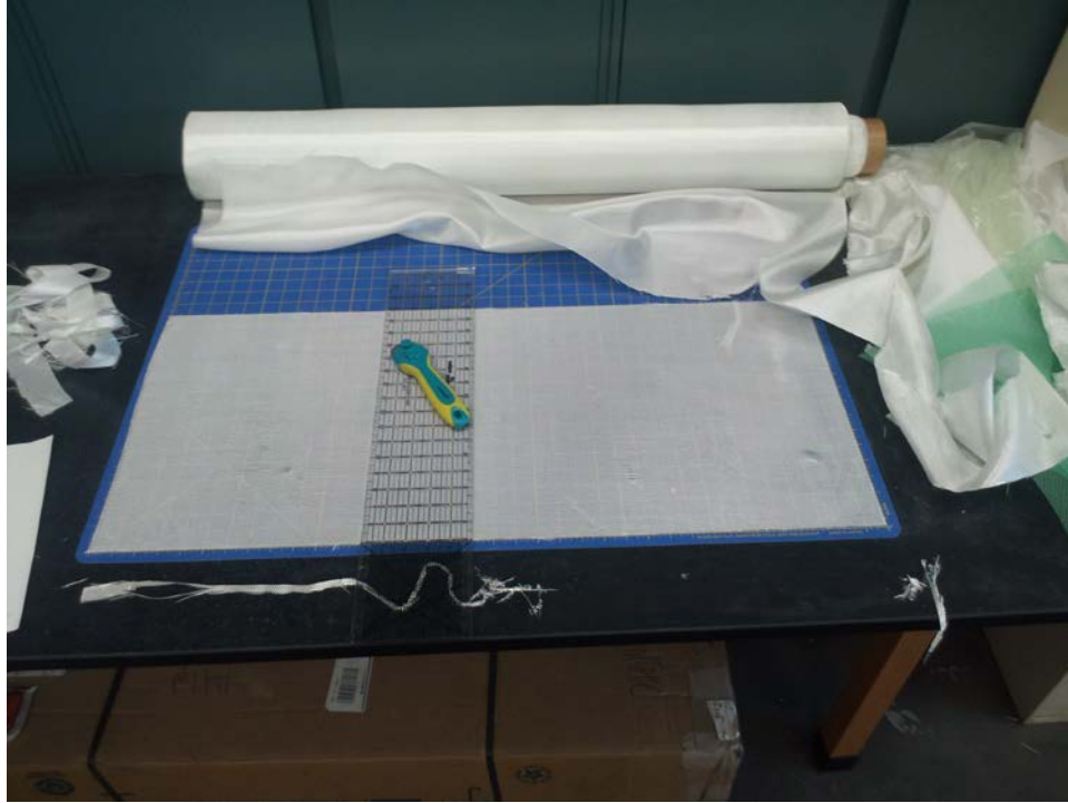
Figure 1. Cutting Layers of E-glass
