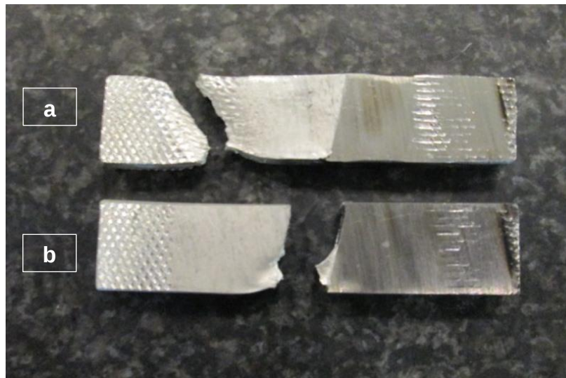
Figure 8 – Tensile Failure of Bimetallic Joint (side view)
