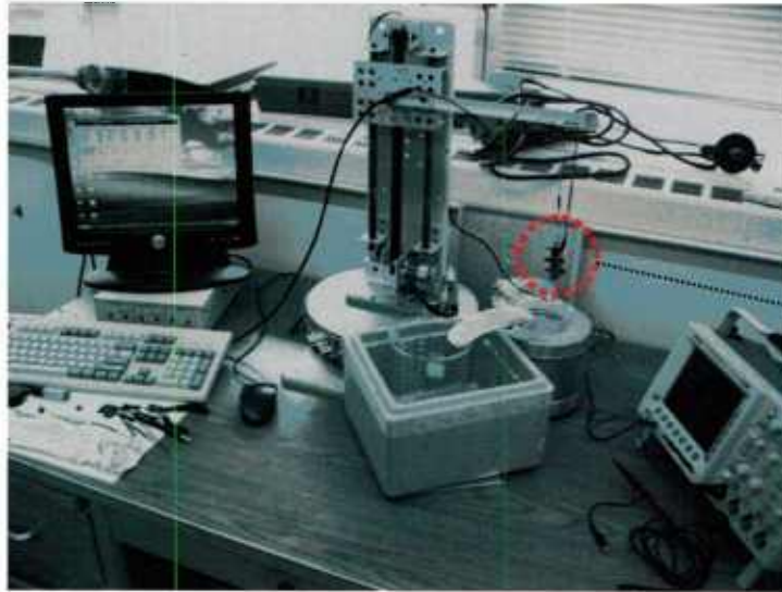
Figure 4.23. Experimental setup, piezo-SMA composite is subjected to thermal cycling
