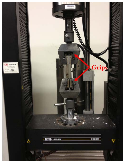
Figure 4.14 Tensile testing setup used for AA1100 and AA5052 specimens.
