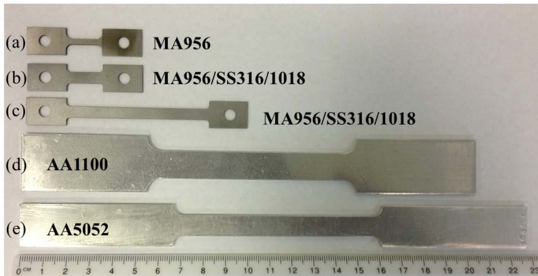
Figure 4.1 Summary of materials and geometries used in this research with corresponding description of use discussed in Table 4.1.
