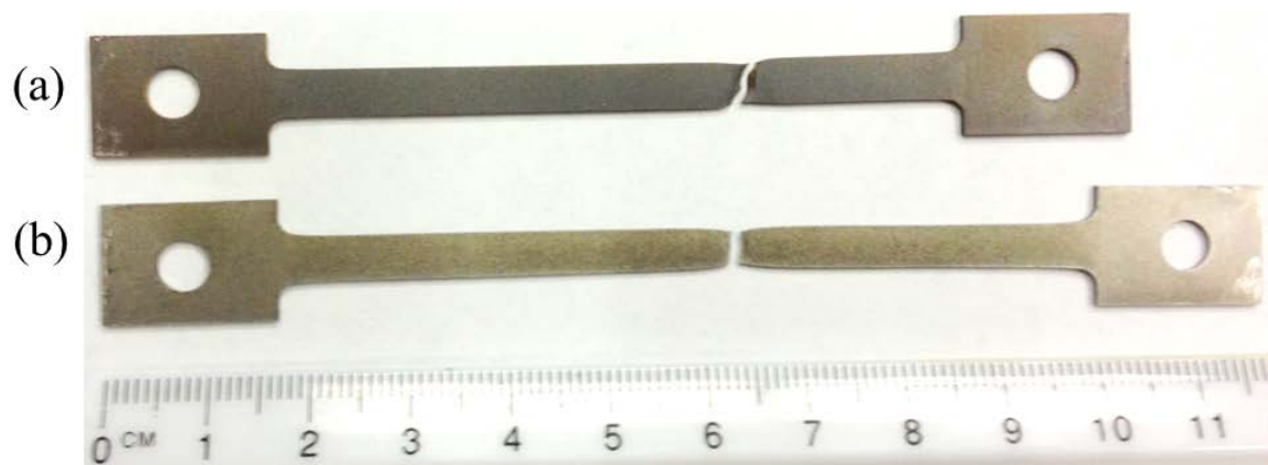
Figure 5.13 Blue brittleness of SS316 for the geometries used in this chapter. Both samples were fractured under identical conditions in air except: (a) 328°C and (b) room temperature.
