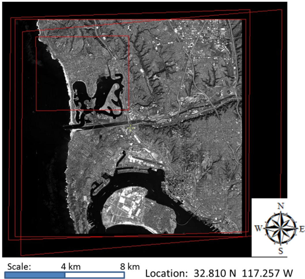
Figure 12. This image shows the large red outline of San Diego WV1 stereo triplet coverage and a smaller interior red box that outlines the downloaded LiDAR coverage for the Pacific Beach area.
