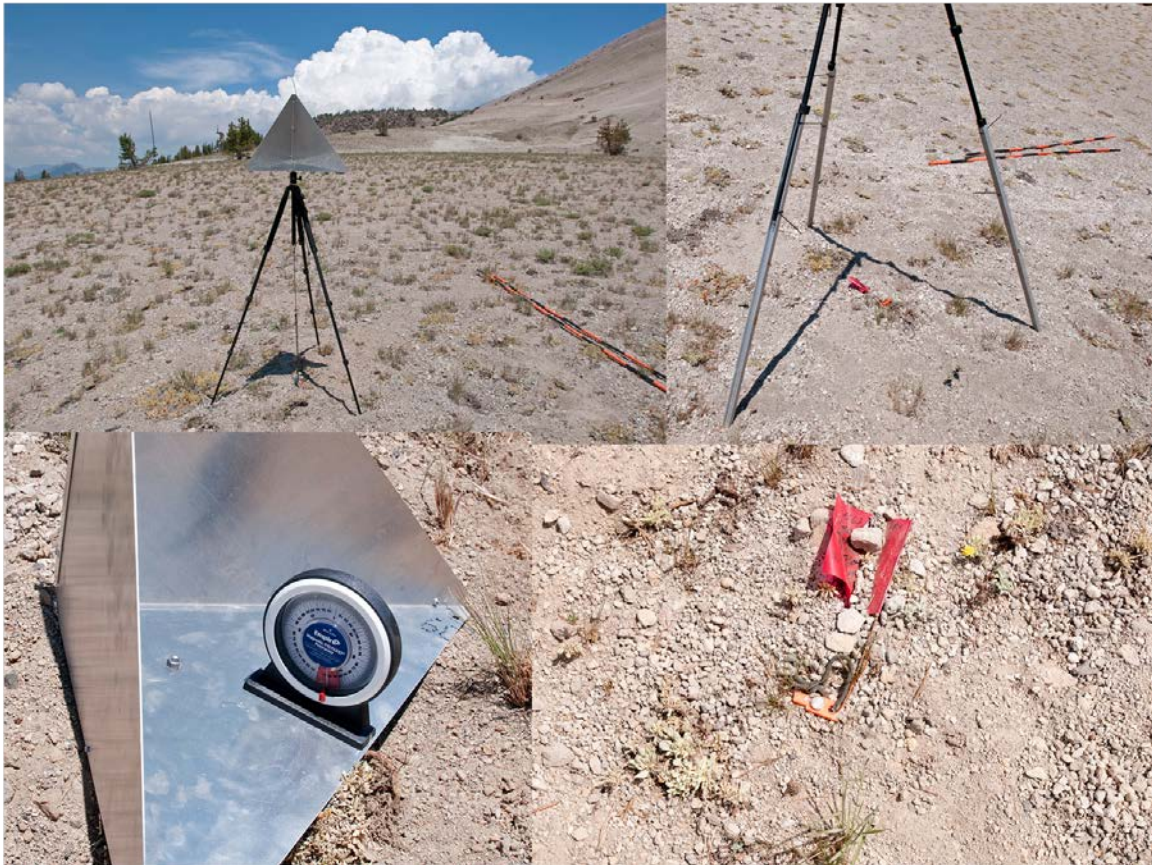
Figure 16. Corner reflector deployment for Snow Off SAR collection.
