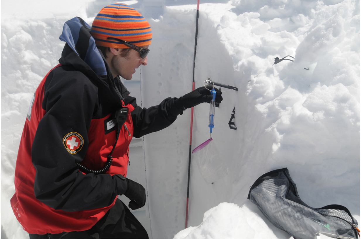
Figure 18. An avalanche snow analysis pit was dug during the SAR collection. A vertical profile of the snowpack's temperature, crystal size, crystal type, and snow density was recorded.
