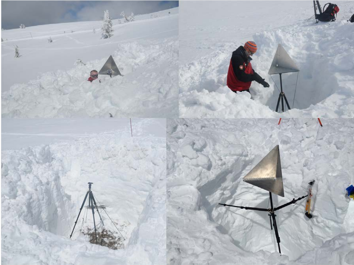
Figure 15. Deployment of corner reflectors used as ground control points at Elysian Fields collection site.
