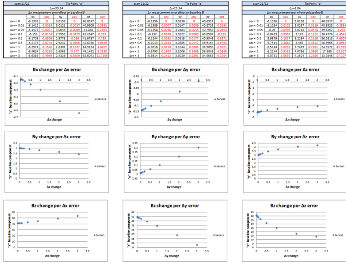
Figure 113. This figure demonstrates the change that the input values of the \Delta x , y , and z elements into the baseline calculation system of equations has on the length of the calculated baseline.
