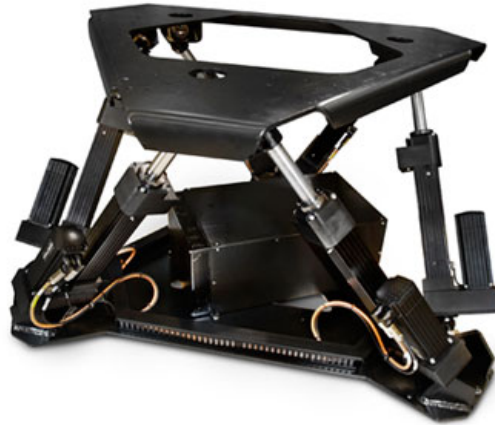
Figure 3. A MOOG 6-DOF motion base similar to the one used in this study
