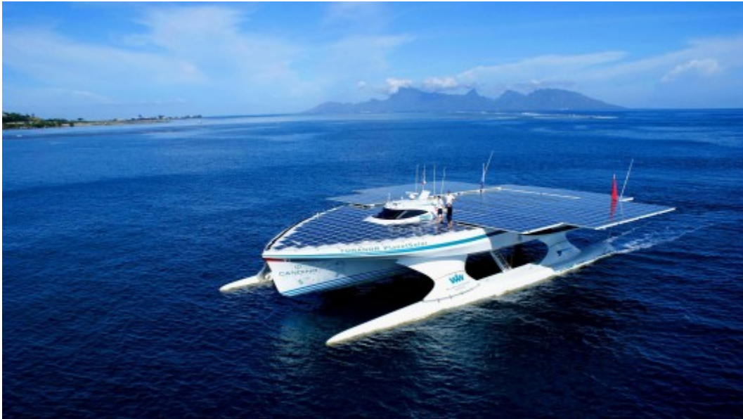
Figure 2. The completely solar-powered yacht TURANOR PlanetSolar . From [3]
