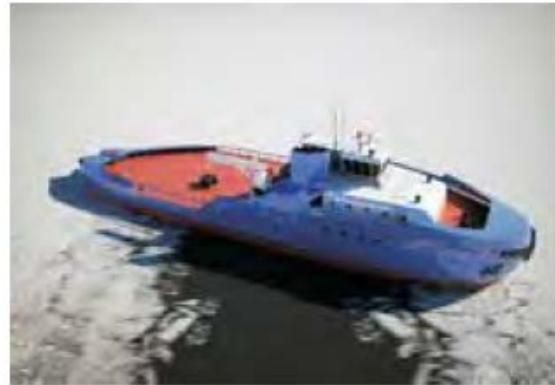
Figure 10. Oblique (Three Podded) Ice Breaker From [8]
