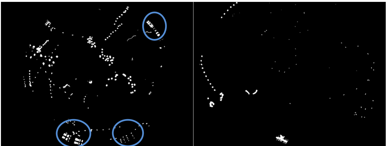
Figure B-4. Epifluorescent "Motion" Images. The motion image on the left was collected from a sample well on a sample well tray (with chamber wall reflections circled in blue ellipses). The image on the right was collected from an unruled Sedgwick Rafter counting chamber. Note there are no wall boundary effects (such as residual signals or multiple organism reflections) observed in the unruled Sedgwick Rafter counting chambers. Also note that organisms that swim into or out of the field of view are "tracked" by the automation algorithms.
