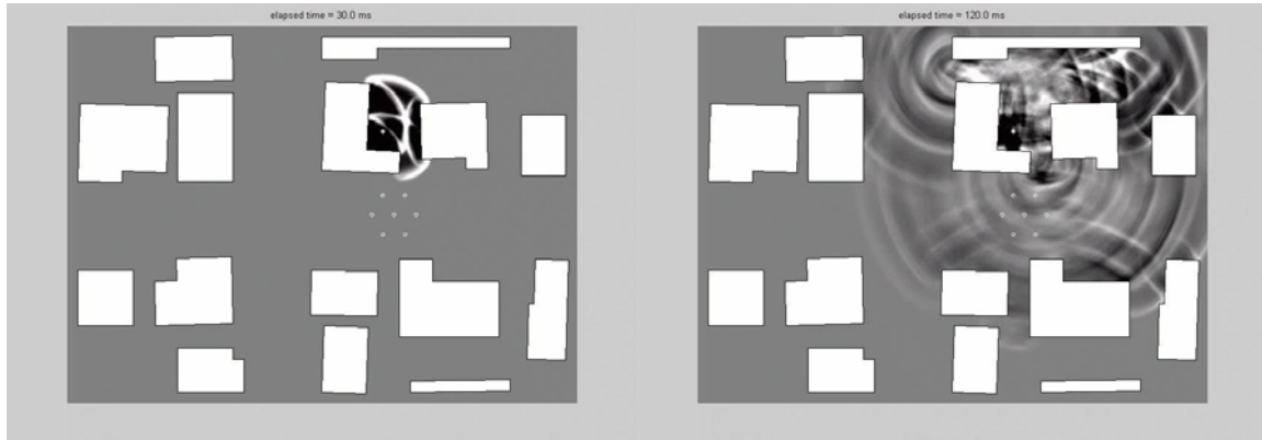
Figure 8. Calculated acoustic pulse propagating from a point source at a different location from previous examples.
