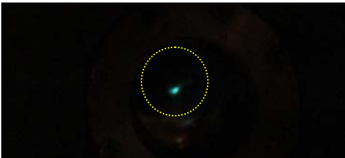
Figure 6: A picture showing the phosphor screen anode of the imaging detector. The green-blue spot corresponds to the detection of neutral atoms created from collisional detachment of stored ions with those few residual gas molecules that remain in the common straight section
