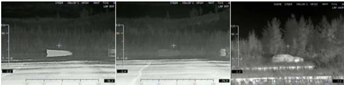
Figure 4. The picture at left shows a vehicle with no ADAPTIV system; the middle picture shows the effect of the concealment through ADAPTIV; and the right picture shows the capability of the ADAPTIV system for deception as it simulates the signature of a car.
