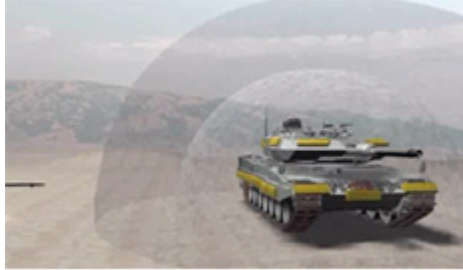
Figure 6. German ADS system with incoming missile and ranges for detection (dark grey) and destruction (light grey).
