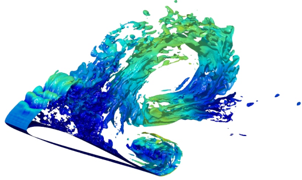
Figure 3: Splitting of the mesh around an SD7003 airfoil into implicit and explicit elements. Less than 9% of the elements are in the boundary layer and integrated using the implicit scheme. The right plot shows an instantaneous flow solution, as isosurfaces of the entropy colored by the Mach number.
