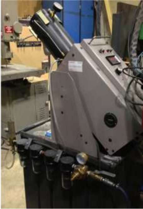
Figure 6, Mass erodant particle flow controller
