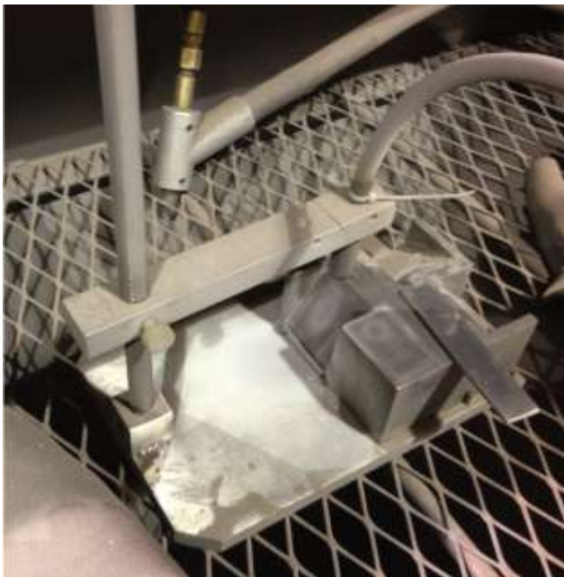
Figure 7, Erosion test setup with 30 degree impingement
