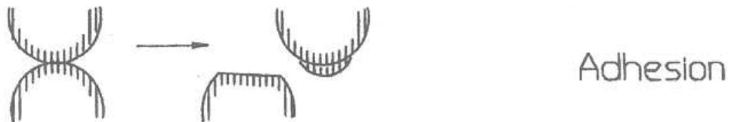
Figure II-3 Adhesive Wear Mechanism [10]
