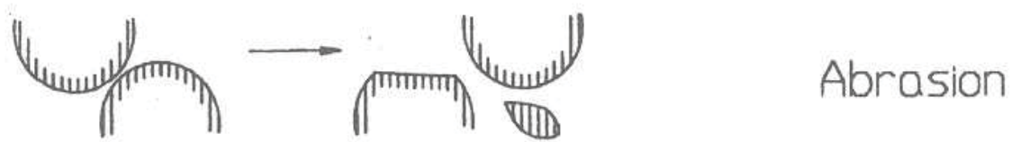
Figure II-1 Abrasive Wear Mechanism [10]
