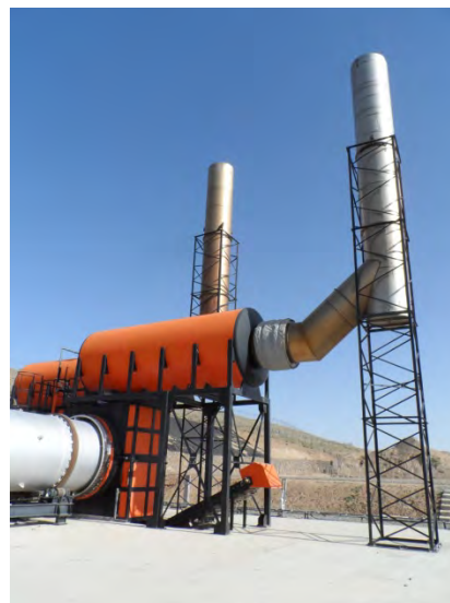
Photo 1 - Two 40-Ton Capacity Incinerators at FOB Sharana
