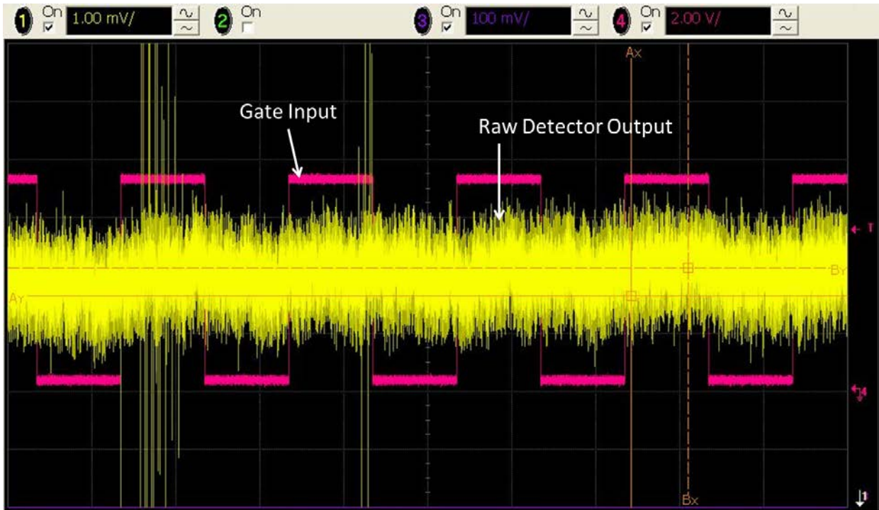
Figure 33. Raw signal from the pyroelectric detector with low power.
