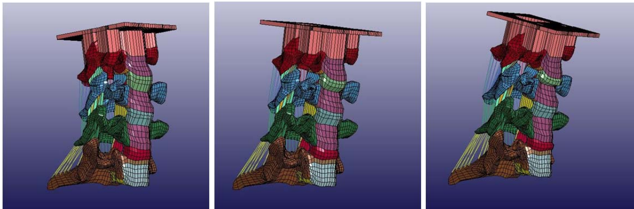
Frontal flexion deformation of LS-DYNA C4-C7 model (moment = 0 Nm; 1 Nm; 2 Nm)
