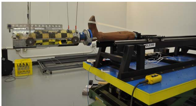
Experimental apparatus for axial lower limb loading; a Hybrid 3 legform is shown.
