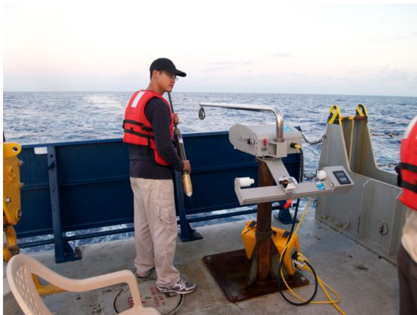
Figure 2. Underway CTD in operation during ITOP. We collected over 3000 temperature profiles of the upper 200 m during the 3-week cruise.
