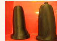
Prepare molds by spraying with demolder
