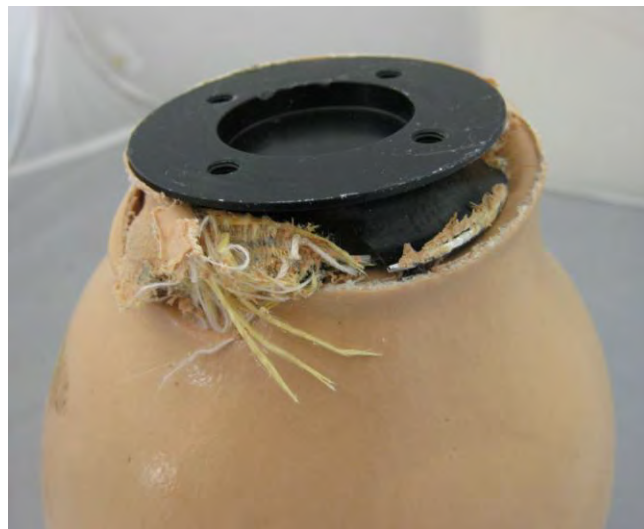
Figure 3: NU-1 distal adapter failure
