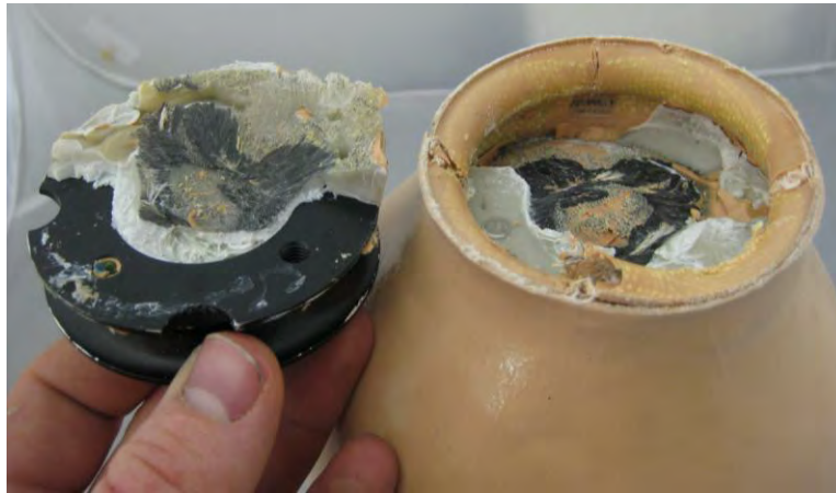
Figure 4: NU-2 distal adapter failure
