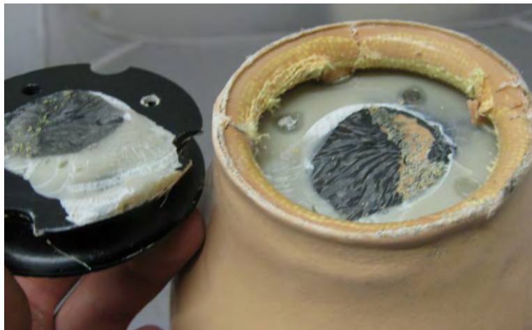
Figure 5: NU-3 distal adapter failure
