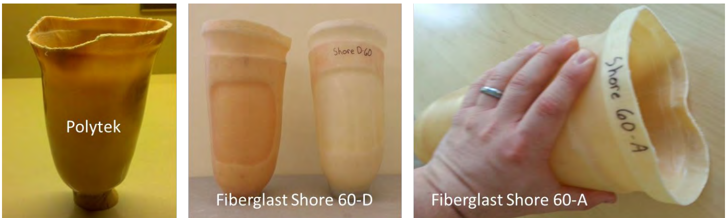
Figure 1 Different socket materials explored as replacements for Polytol.
